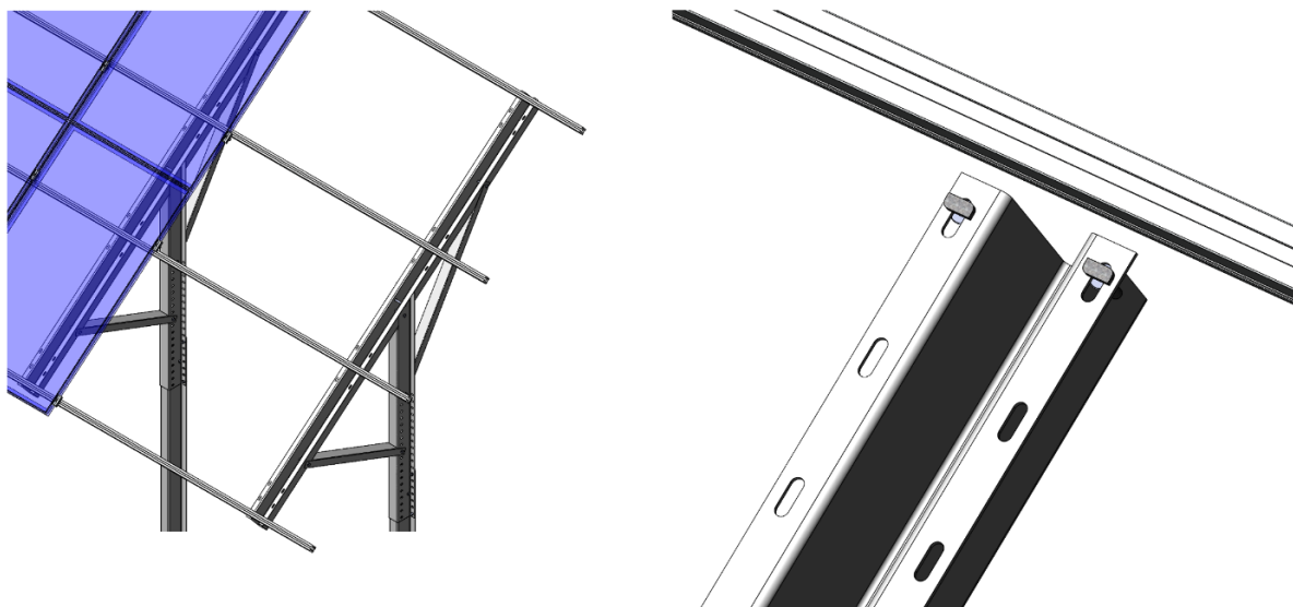
Easy Rail rail attachment to the leg
